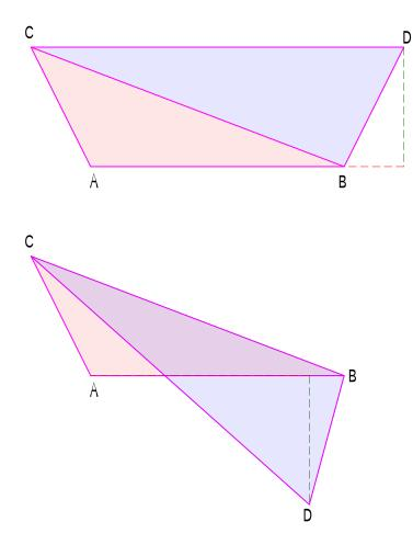
One segment of the **RuleSurf** command result is build out of two triangles or faces. Scanning a mesh in CAD Lisp means in most cases: Start with A and B and calculate C and D, then treat those resulting C and D as a new set of A and B and start all-over, until the complete mesh is processed. In most cases, the first picture is in play. However, sometimes the second picture can be in play. In addition, even C can be under axis AB but focus is on D for proper explanation.
